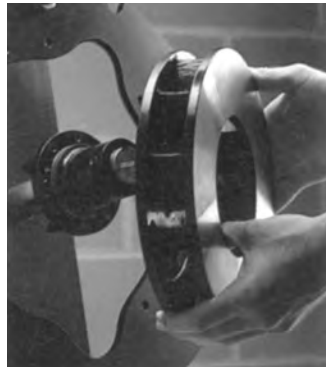
Remove the disc without removing or disassembling the brake.
