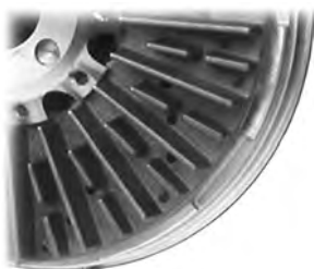
Cross-drilled rotor with heat dissipating fins.
